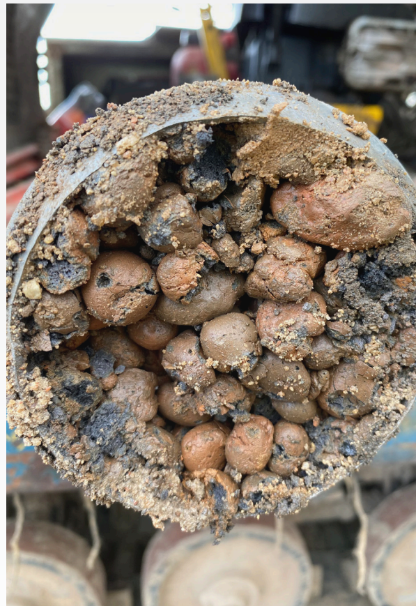
Test sample of Leca LWA taken from the submerged embankment in Varska, Estonia.
