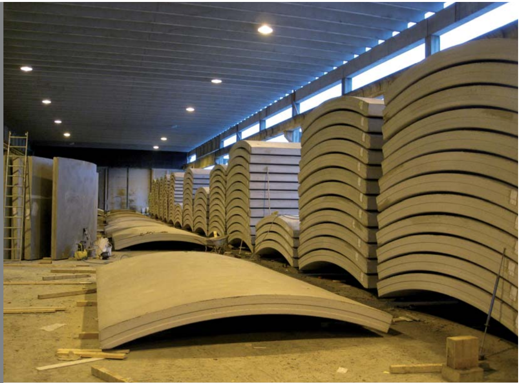
LWAC panels for the Asurtjerne tunnell in norway
