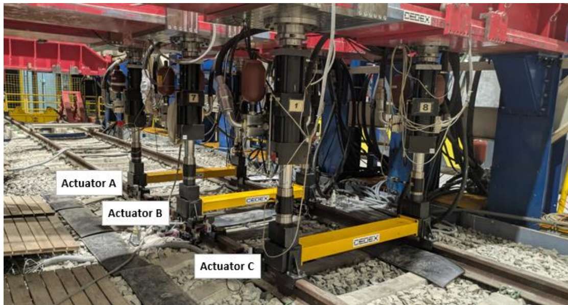
Figure 57.- Hydraulic actuators disposition in CTB
