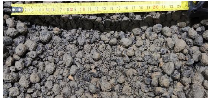
Figure 32.- Left: LECA material at the top of layer, no breakage. Right: LECA material broken at some centimetres below top surface
