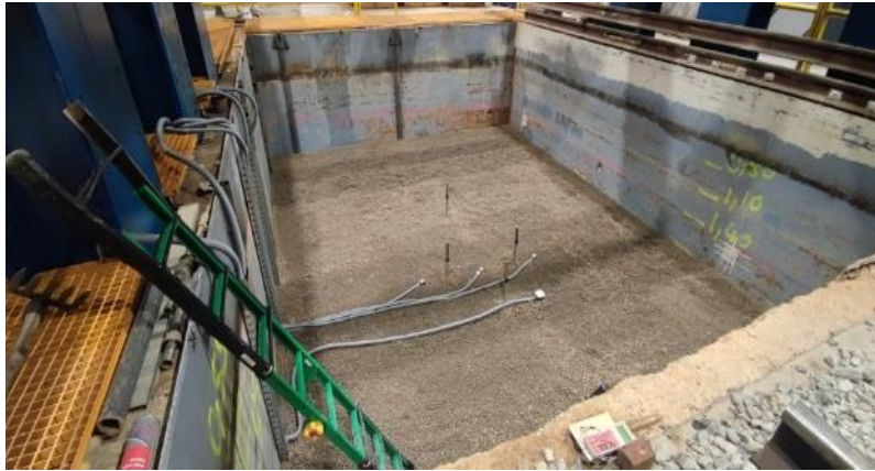
Figure 26.- Left: Aspect of the test section with the half-thickness of LECA embankment, in which some instrumentation was already installed. Right: Execution of Panda test in the half-thickness of LECA embankment. The dynamic load plate is shown in the background
