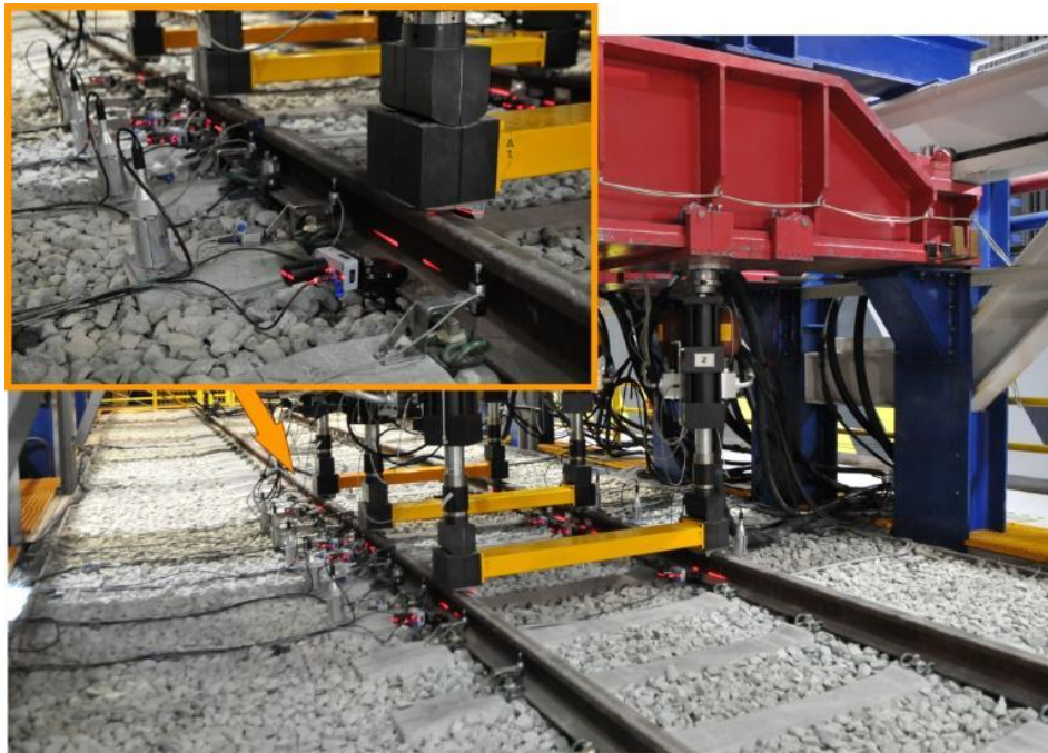
Figure 9.- Surface instrumentation installed in one test
