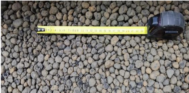
Figure 32.- Left: LECA material at the top of layer, no breakage. Right: LECA material broken at some centimetres below top surface
