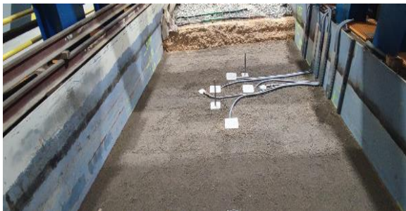
Figure 33.- Left: LECA embankment top with instrumentation. Right: Geotextile over LECA embankment
