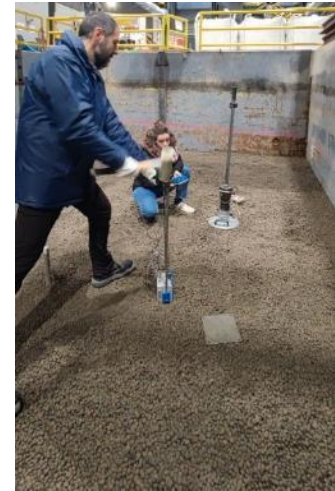
Figure 26.- Left: Aspect of the test section with the half-thickness of LECA embankment, in which some instrumentation was already installed. Right: Execution of Panda test in the half-thickness of LECA embankment. The dynamic load plate is shown in the background
